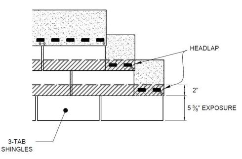
The drawing below shows where the headlap is on 3-tab shingles.
