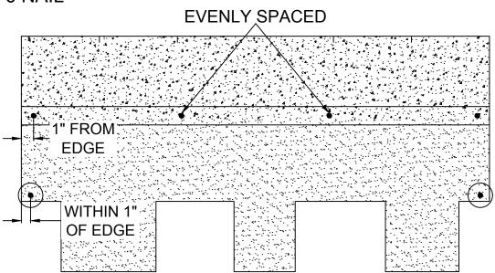
ENSURE FASTENERS IN LOWER NAILING AREA WILL BE COVERED BY TABS OF OVERLYING COURSES
