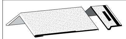
TO CREATE AN EZ-RIDGE STARTER, CUT OFF THE 8  $\chi$ " EXPOSURE PORTION\* OF AN EZ-RIDGE SHINGLE, AND USE THE 3  $\chi$ " REMAINDER (WITH SEAL-DOWN STRIP) AS THE STARTER.
