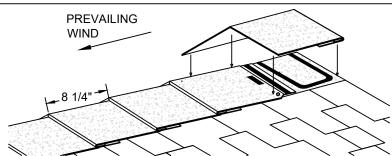
FOR THE LAST SHINGLE OF THE RUN, REMOVE THE CUTOUT END OF THE RIDGE SHINGLE AND TRIM TO FIT, MAINTAINING THE 8  $\frac{1}{4}$ " EXPOSURE. SET THE SHINGLE IN MASTIC.
