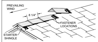
FIRST EZ-RIDGE SHINGLE COMPLETELY OVERLAPS STARTER. POSITION EACH EZ-RIDGE SHINGLE TO FOLLOW WITH AN 8  $\frac{1}{2}$ " EXPOSURE BEFORE FASTENING.
