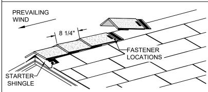
FIRST EZ-RIDGE SHINGLE COMPLETELY OVERLAPS STARTER. POSITION EACH EZ-RIDGE SHINGLE TO FOLLOW WITH AN 8  $\frac{1}{4}$ " EXPOSURE BEFORE FASTENING.
