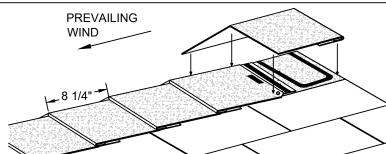
FOR THE LAST SHINGLE OF THE RUN, REMOVE THE CUTOUT END OF THE RIDGE SHINGLE AND TRIM TO FIT, MAINTAINING THE 8  $\mbox{\ensuremath{\mbox{\sc hingle}}}$  EXPOSURE. SET THE SHINGLE IN MASTIC.
