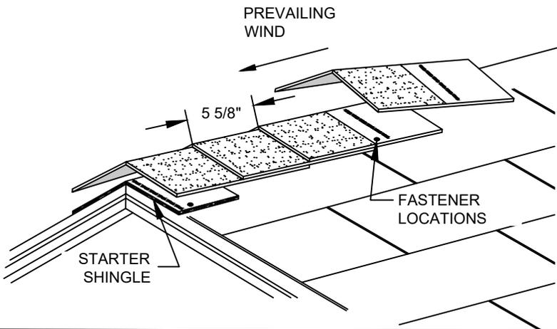
**STARTER:** CUT THE 5 5/8" EXPOSED PORTION OFF A RIDGEFLEX STRIP AND USE THE REMAINING SEAL-DOWN PORTION (7 5/8") AS A STARTER. POSITION WITH SEAL-DOWN AT ROOF'S EDGE, AND FASTEN 3" BACK FROM THE EDGE AND 1" UP FROM THE SIDE.
