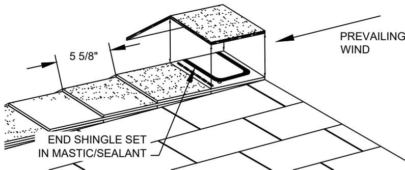
TRIM THE EXPOSED PORTION OF A RIDGEFLEX SHINGLE TO FIT AT THE END OF THE RIDGE, MAINTAINING THE EXPOSURE OF 5 5/8". SET STRIP IN MASTIC/SEALANT.
