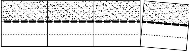
MALARKEY 10" RIDGEFLEX SHINGLES ARE PERFORATED AND SEPARATE INTO FOUR PIECES.
