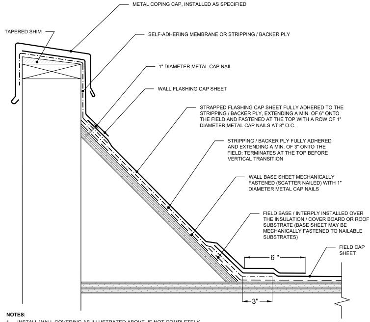
INSTALL WALL COVERING AS ILLUSTRATED ABOVE. IF NOT COMPLETELY WRAPPING THE TOP OF THE WALL, MECHANICALLY FASTEN THE TOP OF THE VERTICAL WALL FLASHING CAP SHEET USING 1" DIAMETER GALVANIZED CAP NAILS, 8" O.C.
