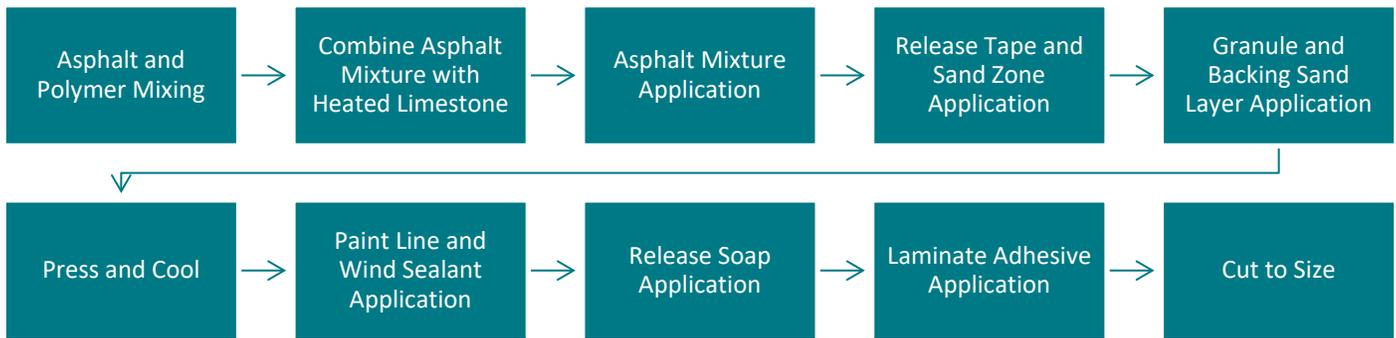
Figure 3 –Shingle production diagram
