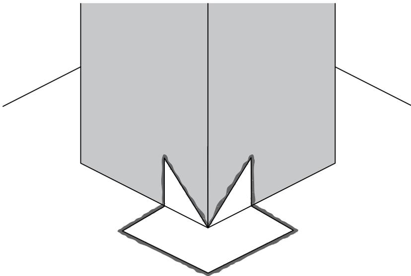
**\* IT IS RECOMMENDED EZ SEAL CORNER REINFORCEMENT BE ALLOWED TO CURE TO A TACKY CONSISTENCY BEFORE PROCEEDING WITH EZ SEAL FLASHING APPLICATION.**
