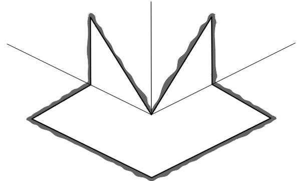
**CLEAN AND ABRABE SURFACES; WIPE WITH ACETONE; INSTALL PRIMER; APPLY EZ SEAL NON-FIBERED PMMA RESIN TO CORNER AND SET 'OUTSIDE CORNER' FLASHING IN RESIN\***
