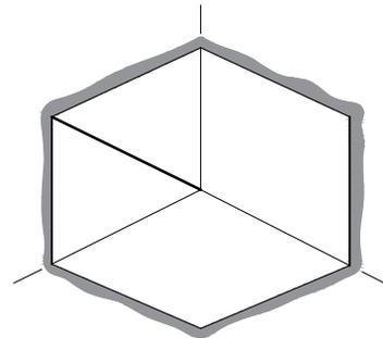
CLEAN AND ABRABE SURFACES; WIPE WITH ACETONE; INSTALL PRIMER; APPLY EZ SEAL NON-FIBERED PMMA RESIN TO CORNER AND SET 'INSIDE CORNER' FLASHING IN RESIN\*
