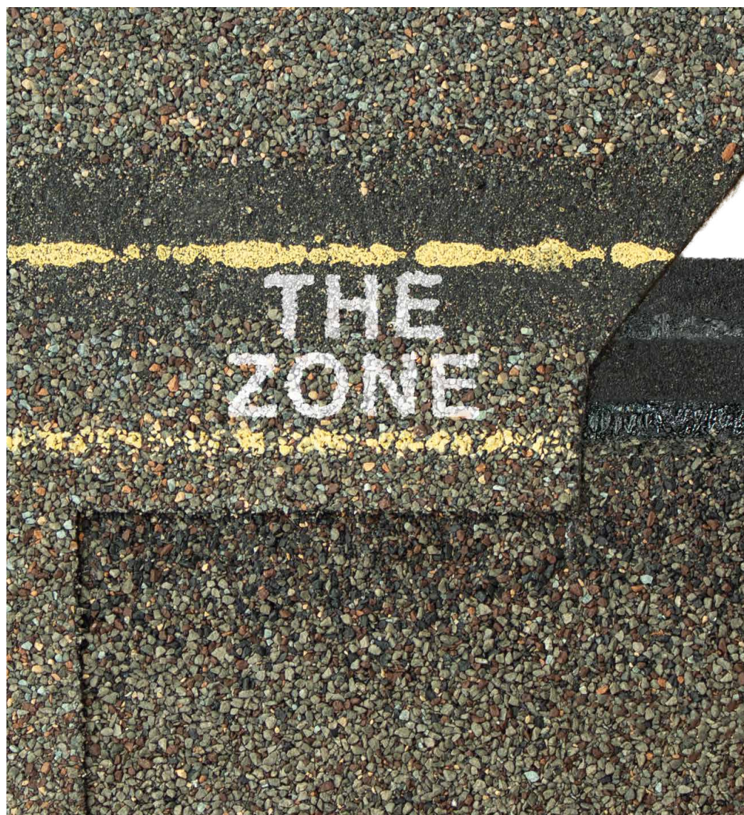
Malarkey Shingle Nailing Area - [1-5/16" wide, 2 rain seals]
