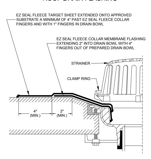
EZ SEAL FLEECE DIMENSIONS DEPEND ON DRAIN DIAMETER CLEAN AND ABRADE SUBSTRATE  $\frac{1}{2}$ " MAX BEYOND EZ SEAL TERMINATION WIPE W/ ACETONE; PRIME PREPARED SURFACE WITH APPROPRIATE PRIMER EXTEND RESIN  $\frac{1}{4}$ " -  $\frac{1}{2}$ " PAST FLEECE
