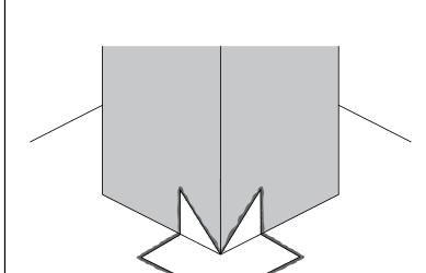
CLEAN AND ABRADE SURFACES; WIPE WITH ACETONE; INSTALL PRIMER; APPLY EZ SEAL NON-FIBERED PMMA RESIN TO CORNER AND SET 'OUTSIDE CORNER' FLASHING IN RESIN\*
