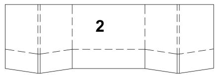
EZ SEAL FLEECE CUT TO MATCH SUBSTRATE/PENETRATION ANGLE
