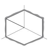
CLEAN AND ABRADE SURFACES; WIPE WITH ACETONE; INSTALL PRIMER; APPLY EZ SEAL NON-FIBERED PMMA RESIN TO CORNER AND SET 'INSIDE CORNER' FLASHING IN RESIN\*
