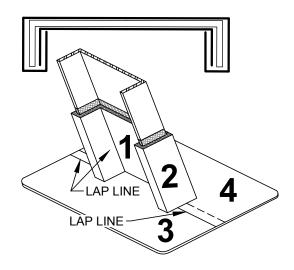
ALL FLEECE-TO-FLEECE LAPS REQUIRE ADDITIONAL EZ SEAL NON-FIBERED PMMA RESIN BASE COAT BETWEEN FLEECE LAYERS
