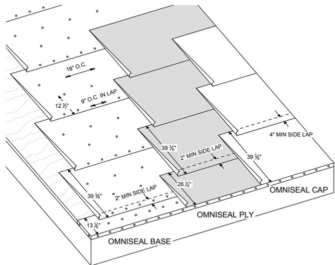
**Figure 1 - 3-Ply Layout of OmniSeal™ Membranes (Drip Edge Not Shown for Clarity)**
