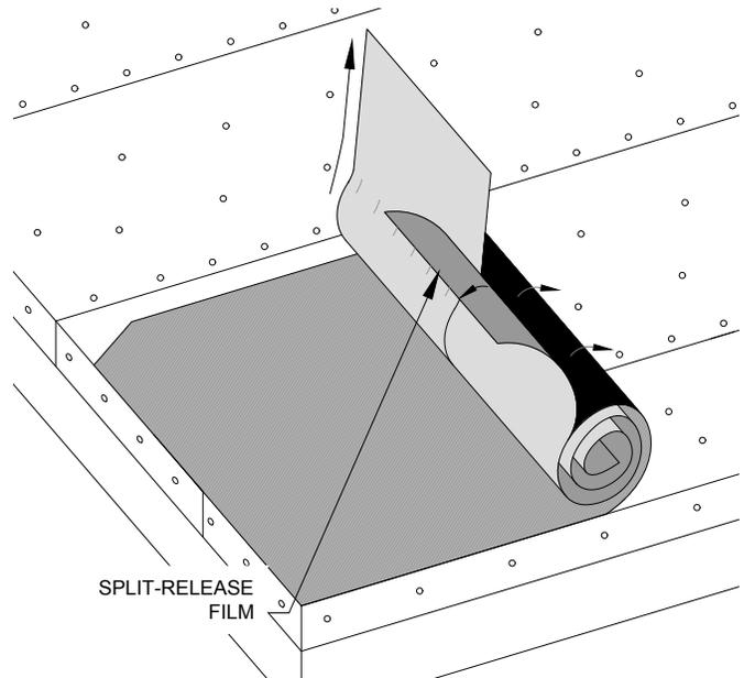
**Figure 5 - Application Technique in Elevated Temperatures**
