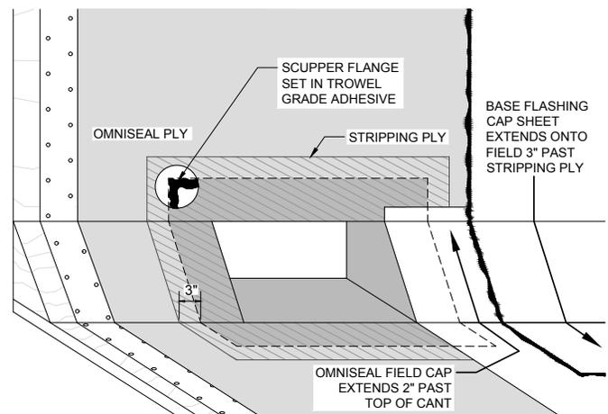
**Figure 11 - Application of the OmniSeal™ System at Scuppers**
