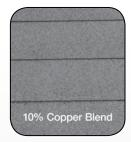
Grey scale images showing black streaks caused by algae growth on shingles exposed in Houston, TX for 5 years. Shingles with low blend percentages show significant discoloration already.
